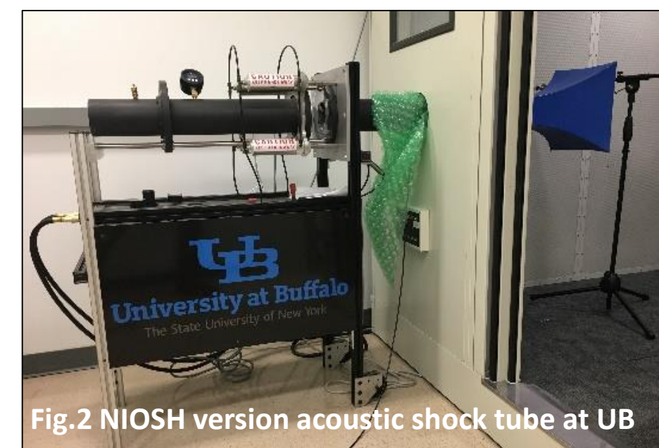
Fig.2 NIOSH version acoustic shock tube at UB
